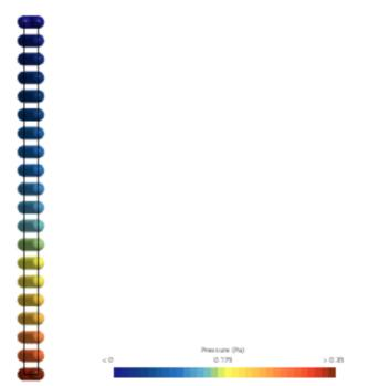
This plot shows the pressure in the flow channel along y. The pressure starts at 0.35 Pa at is 0 Pa at the end.
