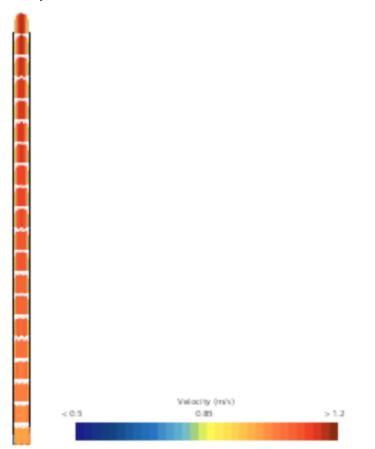
The velocity distribution at the inlet is equal across x and as the flow progresses through the channel the flow forms a parabola but the velocity at the center is still generally equal. The parabola formed here is much less defined than that of the laminar flow.
