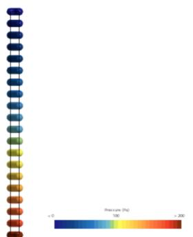
This plot shows the pressure in the channel as it ranges from 200 at the inlet to 0 at the outlet. The pressure gradient in this simulation is much higher than that of the laminar regime.
