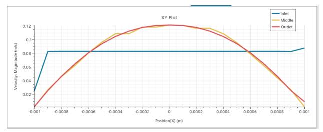
The velocity plot shows that the fluid enters the heat exchanger in plug flow, approximately reaches laminar flow in the middle, and has fully developed by the outlet. This is indicated by the parabola which is indicative of fully developed laminar flow.
