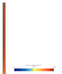
This plot shows the velocity development from plug flow to laminar flow with no-slip boundary conditions. The velocity at the inlet is all at the same velocity, plug flow, and develops to a parabola at the outlet, fully developed laminar flow. The velocity is greatest at the middle and lowest at the walls.
