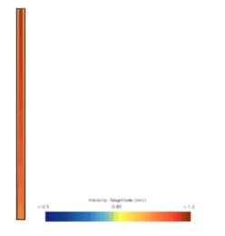
The turbulent flow remains even across x for a long time but eventually begins to form a parabola like in the laminar simulation. The flow is again fastest in the center and slowest at the walls.
