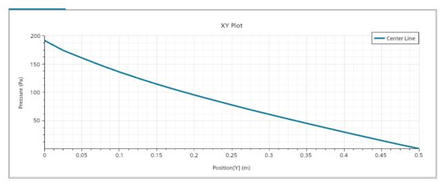
This plot is the pressure down the centerline. It looks similar to the laminar pressure plot but the gradient is much greater. The plot is again approximately linear like the laminar flow plot.
